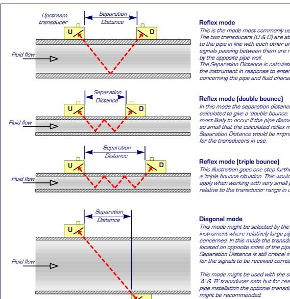
This is the mode most commonly used. The two transducers (U & D) are attached to the pipe in line with each other and the signals passing between them are reflected by the opposite pipe wall.
